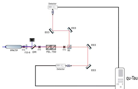
Figure 11. Temporal correlations experimental setup to study the time delay between the signal and idler photons.
