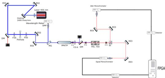
Figure 16. Joint Spectrum setup. signal and idler photons are sent to monochromators, where only specific values of wavelength pass through and into multi-mode fibers for the single photon counters. A count of coincidences at  $\lambda_s$  and  $\lambda_i$  takes place and is plotted as an intensity in the joint spectrum
