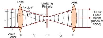
Figura 6. spacial filter. First lens focuses light into pinhole to clean the pump beam from noise. Second lens is used to focus light beam into the posterior setup.
