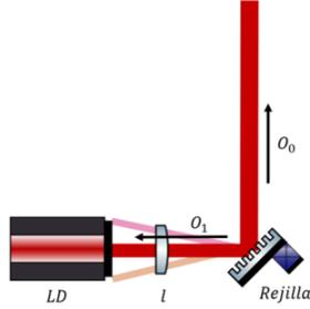
Figura 4. Littrow configuration setup design. Image taken from [9].
