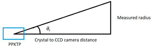
Figure 17. Triangle formed by pump wave and signal wave. The radius of the ring is measured in pixels and converted to distance. In the CCD Camera, one pixel corresponds to  $9 \mu\text{m}$ .
