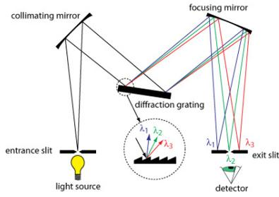
Figure 13. Illustration of the functioning of a monochromator. Incident light with multiple frequencies gets dispersed by a grating of 800 lines/mm so that a desired wavelength is not filtered out. The grating may be rotated to measure any wavelength within the specified domain. Image taken from <https://asdlib.org/imageandvideoexchangeforum/wavelength-selection-using-a-monochromator/>
